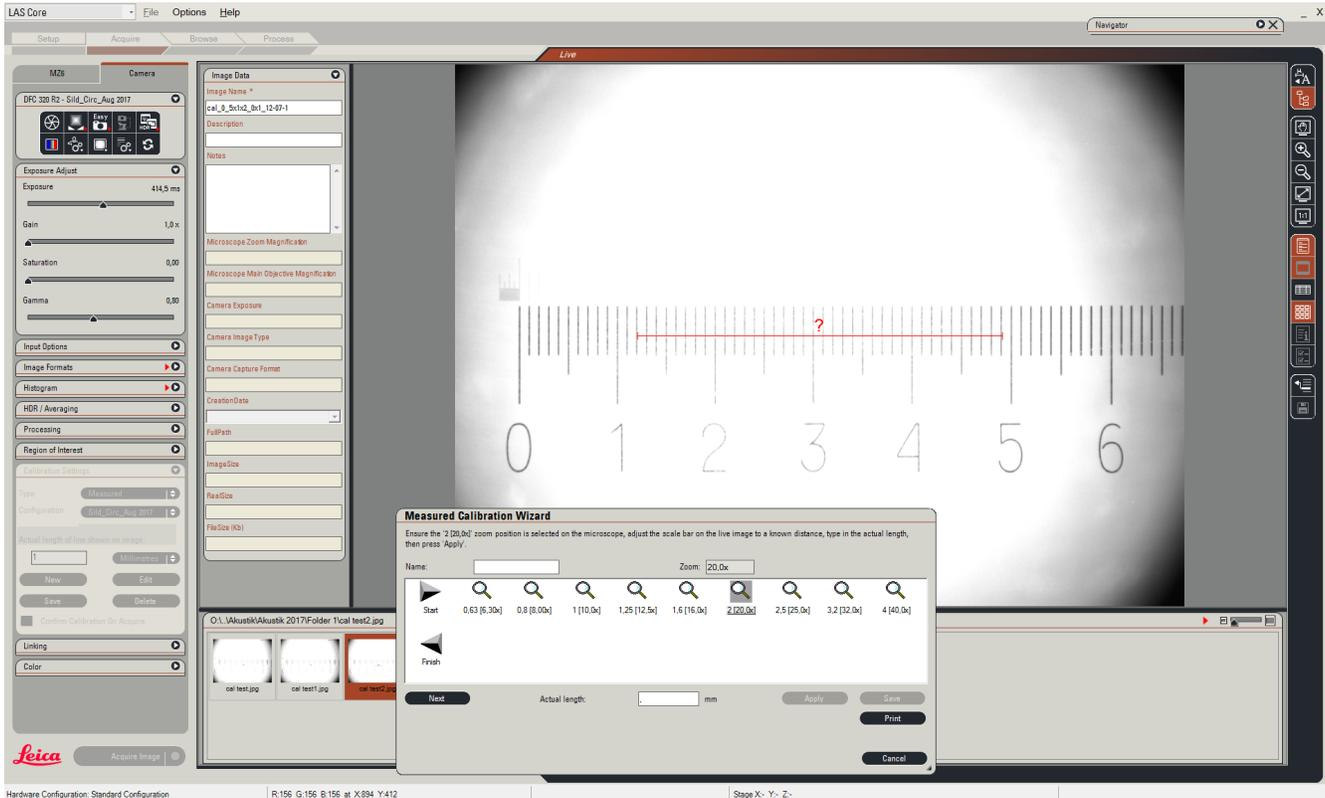
1. Using the 5 cm measuring stick focus the image until it is sharp and marks appear clearly in the image viewer.
